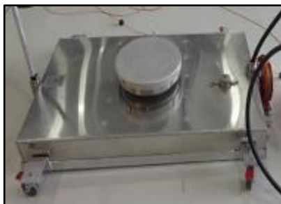
TAD-NH90MRH90-FDS-01 NSN 2910-66-164-7796 Fuel Drain System
