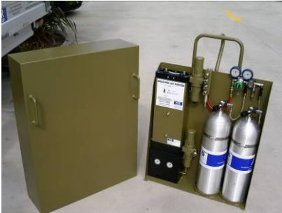
1) Air Test Kit Testing Breathing Air Quality 2) Dew Point Kit Measuring the moisture content in the air.
